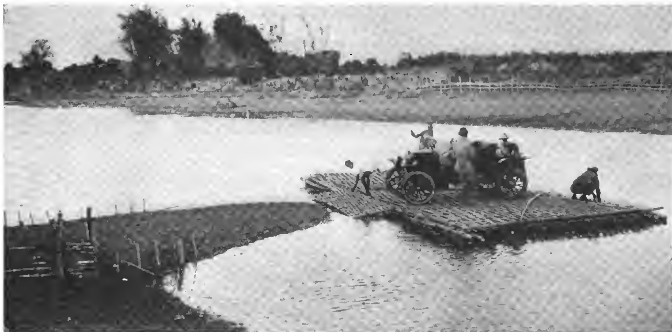
A typical bamboo ferry. Many have disappeared of late years but there are some still left. The carrying capacity of bamboo is very great. For example, the world-touring Hupmobile the first car to make the 175-mile trip from Manila to Baglio, crossed here on a raft of thirty 4-in. bamboo poles
